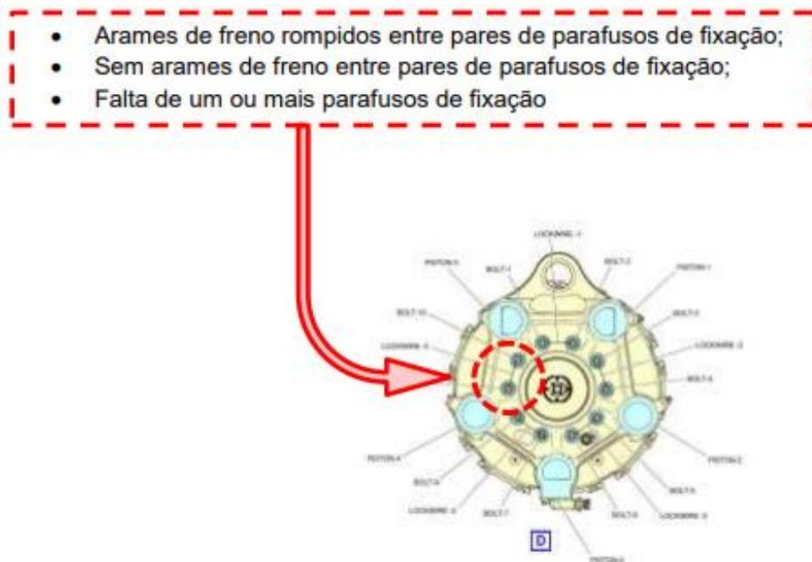
Fonte: Service Bulletin Embraer IB 190E2-32-0001 -LANDING GEAR – BRAKE ASSEMBLY PN 2-1768 WITH LOOSE/MISSING BOLT AND/OR BROKEN LOCKWIRE (2020).
